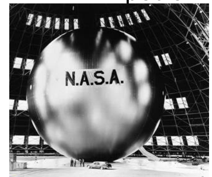
Static Inflation Test of 135 Ft Satellite in Weeksville, NC NASA Langley Research Center Image # 1996-00009
