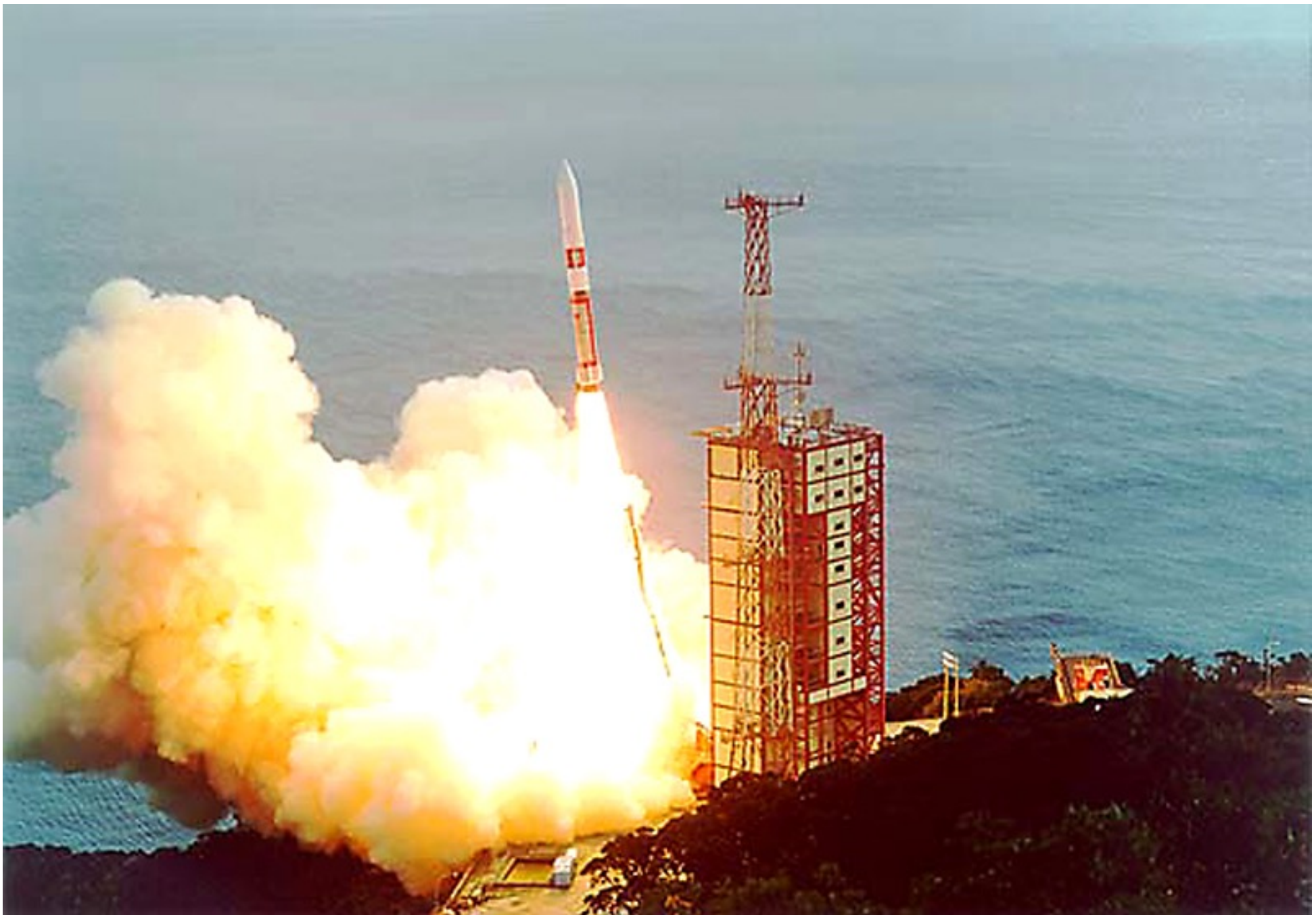
Launch of Haruka on board of a M-V rocket VLBI space observatory program
