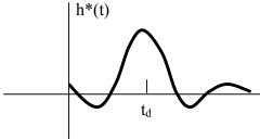
However, such a manipulation will distort  $H^*(t)$ . Distortions could be minimized if  $t_d$  is increased. For practical purposes, if  $t_d \sim 2$  to 3 times  $\pi/\omega_s$ , then  $h^*(t)$  is a close version of h(t). In radio technology, there are three examples of low-pass filters that minimize distortions and have principally different characteristics.
