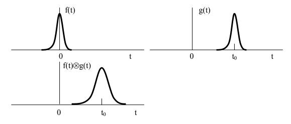
Determining the lag or time delay between signals is for instance used in radio interferometry. An exact determination of the delay,  $t_0$ , will lead to an exact determination of the position of an object in the sky provided the baseline vector,  $\mathbf{B}$ , is known.
