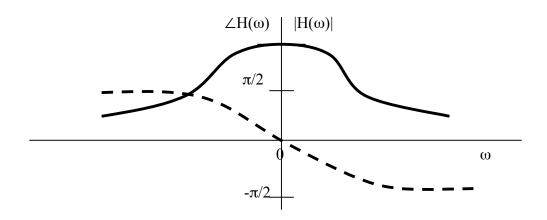
Obviously, a low-pass filter has characteristics of distortion-less transmission only for a narrow bandwidth.
