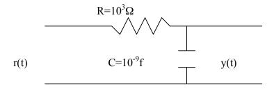
The transfer function of a particular low-pass filter is give by
