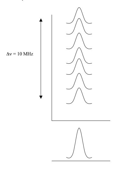
The result is a pulse that is dedispersed – but only to a certain degree. Why? Because the pulse from each filter of the filter bank is still dispersed, only over a bandwidth of 1 MHz as in our example, but still measurable? For instance, in our figure above, the pulse is still a bit smeared out.
