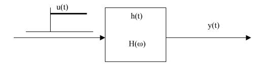
The rise time of the filter is then given by the time it takes y(t) to go from its minimum to its maximum.
