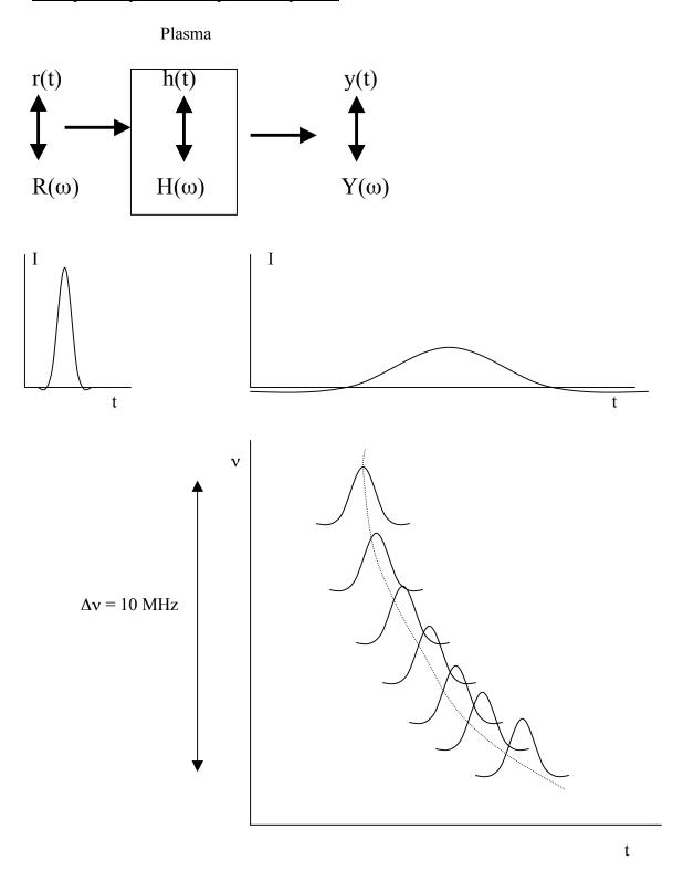
The plasma is dispersive meaning that the phase of its transfer function is a function of frequency,  $\nu$ . That has the effect that pulses emitted at a higher frequency will arrive earlier and pulses at a lower frequency will arrive later. Now suppose that we have a radio antenna with a receiver that has a bandwidth  $\Delta\nu$ , say 10 MHz. Within this bandwidth, the pulse will arrive at a time dependent on frequency. For the ionosphere or
