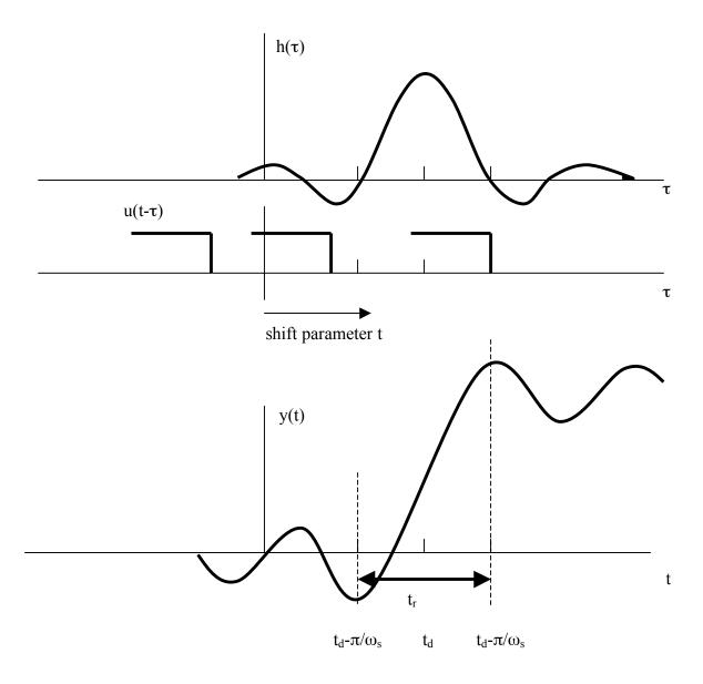
$$\begin{array}{l} t_r{=}2\pi/\omega_s\\ ={1}/{\Delta\nu}\\ Example:~ \Delta\nu=1~MHz\\ t_r{=}~1~\mu s \end{array}$$
