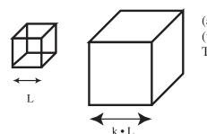
(area)  $A_1 = 6 \cdot L^2$   $A_k = 6 \cdot (k \cdot L)^2$   $A_k = 6 \cdot k^2 \cdot L^2$   $(= k^2 \cdot A_1)$ (volume)  $V_1 = L^3$   $V_k = (k \cdot L)^3$   $V_k = k^3 \cdot L^3$   $(= k^3 \cdot V_1)$ The scaling coefficient is different for area (k<sup>2</sup>) and for volume (k<sup>3</sup>).
