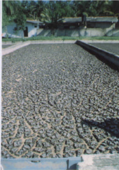
4. Solid waste dries up on the surface of the layers of sand.
