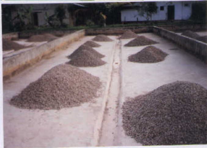
5. Next the dried up particles of solid waste is collected and stored outside.
