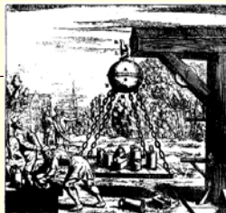
He then hung one hemisphere from a hook and attached a platform to the other hemisphere which he loaded with many heavy weights. The hemispheres still did not come apart.
