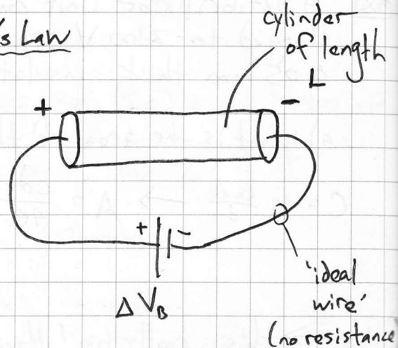
→ battery creates a potential difference  $\Delta V_B$  across the cylinder where  $\Delta V_B = \Delta V_R$  (i.e. the battery creates the voltage drop across the cylinder)
