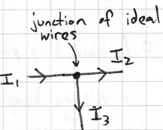
(this stems from the conservation of charge and current; put another way, what flows in must flow out w/ respect to a junction)
