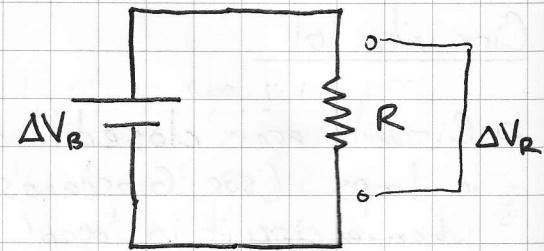
→ battery creates a potential difference across  $R$  ( $\Delta V_R = \Delta V_B$ ) such that electrical potential energy fueled by the battery is 'dissipated' (i.e. burned off) due to the current flowing through it
