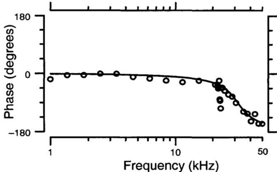
$$\delta(\omega) = \arctan \left( \frac{\gamma\omega}{\omega^2 - \omega_0^2} \right)$$
