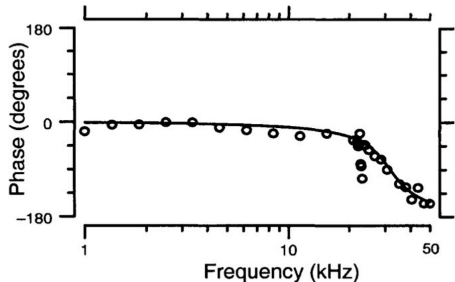
⇒ Characterizing phase slope near resonance provides measure of damping
