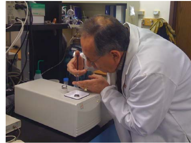
Biophysicist Luis Markey loads his differential scanning calorimetry instrument.
