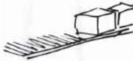
Use roller conveyors to reduce repetitive lifting/handling
