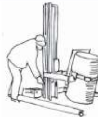
Use specially designed equipment to reduce repetitive handling/carrying
