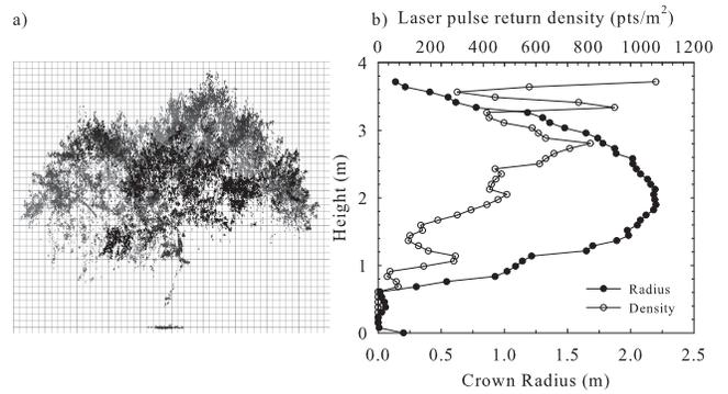
Fig. 3. The measured 3D point cloud data of an olive tree, presented here in a) with an oblique view, can be rapidly analyzed to generate estimates of b) crown profile and pulse return density.
