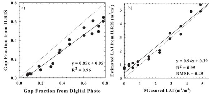
Fig. 2. Laser pulse density retrievals were used to determine a) gap fraction of the artificial tree for 10 stages of crown foliage density. Gap fraction from ILIRIS data are compared with retrievals from estimates from digital photography. In addition, b) Leaf Area Index estimates from the laser pulse data, show close agreement with measured values, taking into consideration leaf angular distribution.
