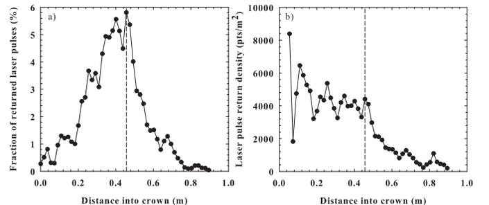
Fig. 1. Segmentation of the XYZ points ( $n = 48,876$ ) of one ILRIS 3D scan into slices with a thickness of 2cm yields (a) laser pulse distribution as function of crown distance, as well as (b) the pulse return density with the appropriate determination of crown area. Dotted line indicates stem location
