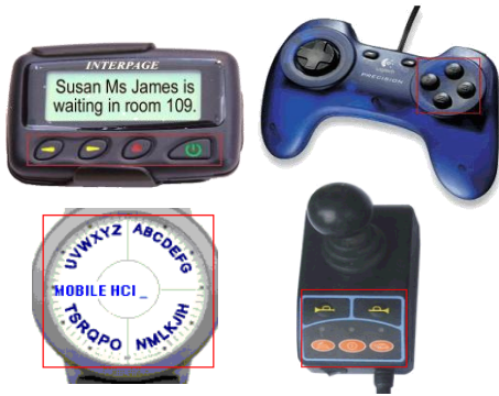
Figure 2. Devices with very few keys or buttons. The Dunlop [7] watch interface is shown in the lower left.
