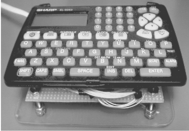
Figure 3 - The modified Sharp EL-6053 , showing the circuit board and protective cover underneath the keyboard
