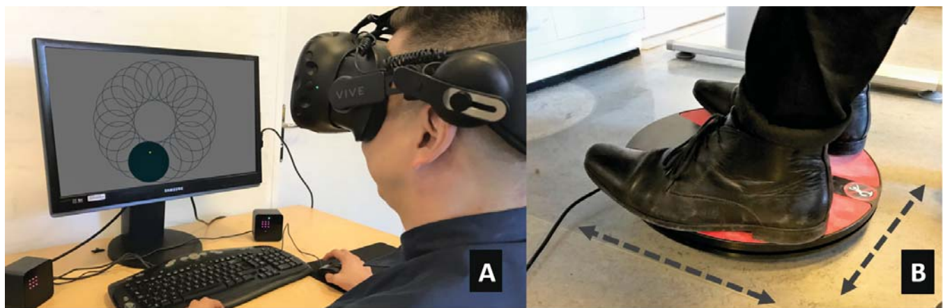
Figure 1: (A) HTC VIVE head-mounted display (HMD) equipped with the Pupil Lab's binocular gaze tracking unit was used for gaze input. The Fitts' law multi-directional selection task that the participant sees inside the headset is shown on the monitor. The headset tracks orientation when used for head input. (B) A 3DRudder foot mouse with 360° movement control was used for foot input. Tilting the 3DRudder moves the cursor in the tilt direction.
