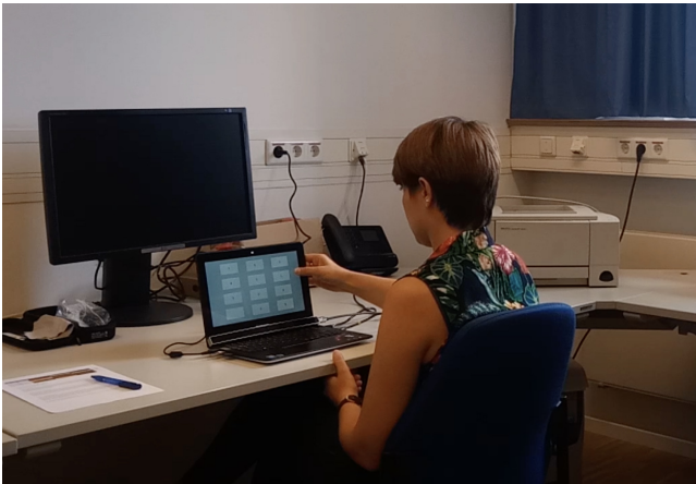
Figure 3: Experimental setup: A participant performing the experiment using TouchGazePath on a laptop computer equipped with a touch-screen and an eye tracker.
