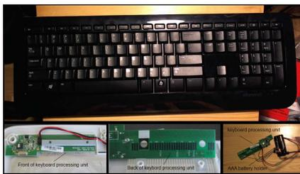
Figure 2. Microsoft *Wireless Keyboard 800* and the keyboard-processing unit.
