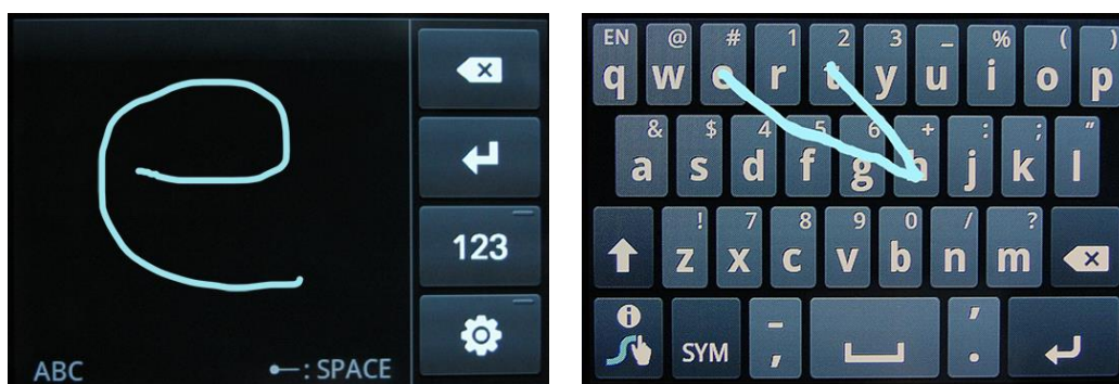
Fig. 2. The letter “e” being entered using DioPen (left). The word “the” being entered on the Swype keypad (right).
