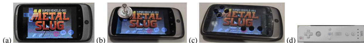
Fig. 3. Input methods used in the study. (a) Soft gamepad. (b) Nano-stick. (c) Foam buttons. (d) Wiimote .
