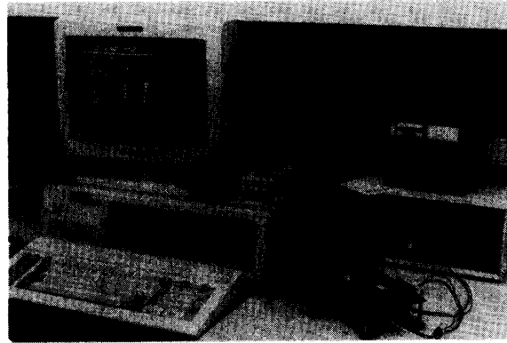
Fig. 3. A typical PC-based development system. Note the EPROM programmer on the system chassis with a ribbon cable connecting to an interface card inside the system. A single-board computer connects to the PC serial port via an RS-232C cable.
