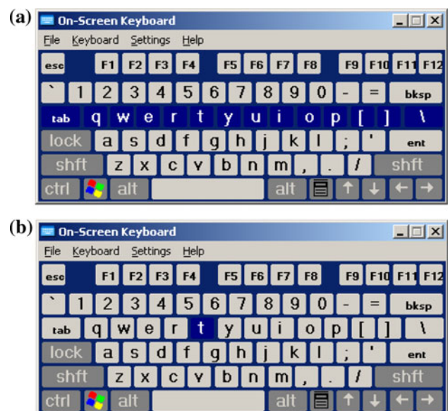
Fig. 4 Scanning keyboard in Microsoft Windows XP a scanning is at the third row, b scanning is at the sixth key (“t”) in the third row
