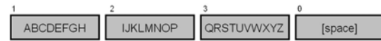
Fig. 7 SAK alphabetically ordered letter arrangement yielding the lowest scan steps per character ( SPC = 1.713 )
