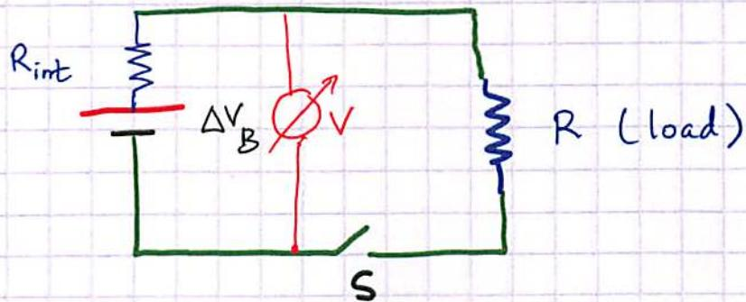
Before  $S$  is closed: Voltmeter is very good, requires almost no current to measure  $\rightarrow$  voltage drop across  $R_{int}$  is negligible  $\rightarrow \Delta V_B$  is displayed!
