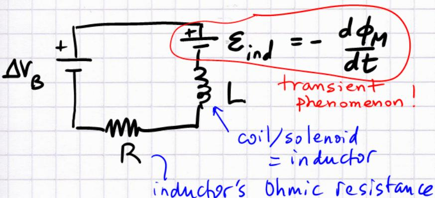
As with the Ohmic resistance of the coil we put the self-induced EMF in series with the coil
