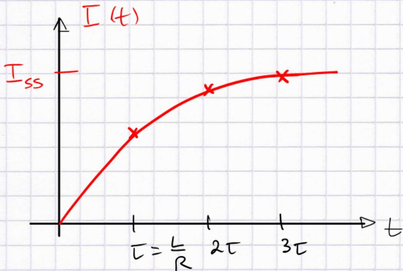
When we close the switch in any circuit, especially in circuits with a coil or solenoid (electromagnet) : the current cannot turn on instantly, it builds over time. The time constant is  $\tau = L/R$ .
