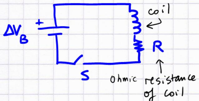
Assume there is no magnetic flux through the coil (earth's field and other magnets present in the lab are shielded)
