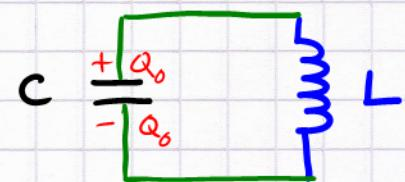
At  $t=0$  no current flows, but there is an  $\vec{E}$  field, i.e., electrical energy in the capacitor.  $C$  starts discharging by attempting to pass a current through  $L$ .
