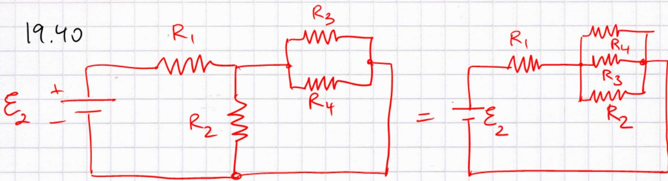
$$\therefore R_{\text{tot}}^{\text{eq}} = R_1 + R_{234}^{\text{eq}}$$
