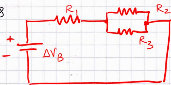
$$R_{23}^{eq} = \frac{R_2 R_3}{R_2 + R_3}$$
