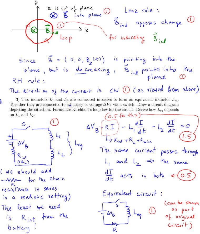
$$\Delta V_{B} - RI - L_{1} \frac{dI}{dt} - L_{2} \frac{dI}{dt} = 0$$
