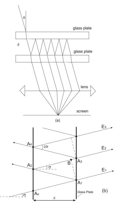
Figure 1: (a)Fabry-Perot setup (b) Fabry-Perot cavity.
