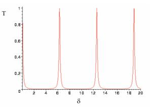
Figure 2: Transmittance as a function of phase, r = 0.95.
