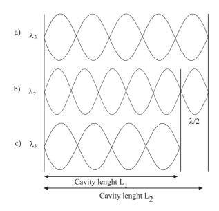
Figure 4: Change of one free spectral range.
