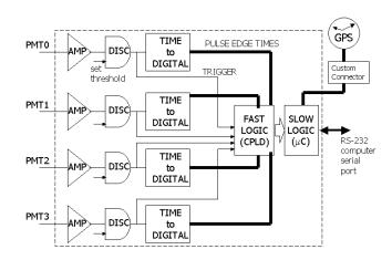
Fig. 3. Hardware block diagram (Version 2).
