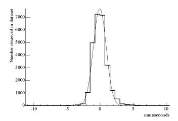
Fig. 4. Histogram of measured time differences between leading edges of pulses from two counters in contact, from a muon telescope experiment at the University of Washington. Actual time differences should be on the order of a few ps. The fitted Gaussian has 1 ns standard deviation, consistent with TMC resolution.
