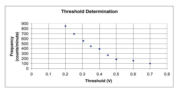
Figure 80. A graph of frequency vs. threshold for a counter used to determine threshold setting.
