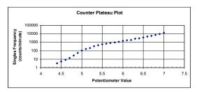
*Figure23. Example of counter plateau graph used to determine operating voltage of PMT.*
