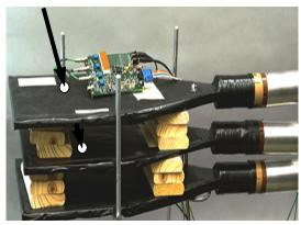
*Figure20. A three counter muon lifetime detector system.*
