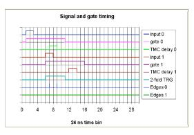
*Figure36. Signal and gate timing diagram for Example C.*
