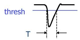
Figure 5. Typical PMT pulse from which the Time Over Threshold (TOT) can be determined.
