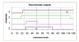
Figure 38. Discriminator output timing diagram for Example D.
