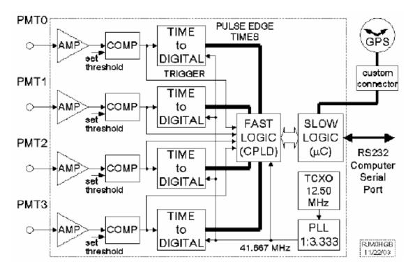
Figure 4. Block diagram of the QuarkNet DAQ v2 board.
