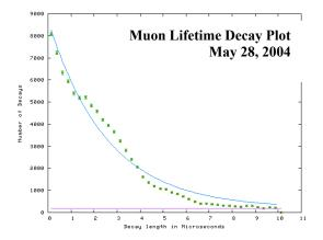
Figure 21. A lifetime graph showing number of number of decays as a function decay from when the muon entered the scintillator. Fitting this data to an exponential decay function can yield the lifetime.
