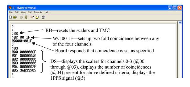
*Figure27. A sample terminal emulation window displaying how to set coincidence levels and how to read this coincidence data.*
