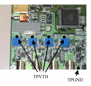
Figure 7. Close-up picture of the DAQ board showing threshold test points used to measure threshold voltage for each channel.
