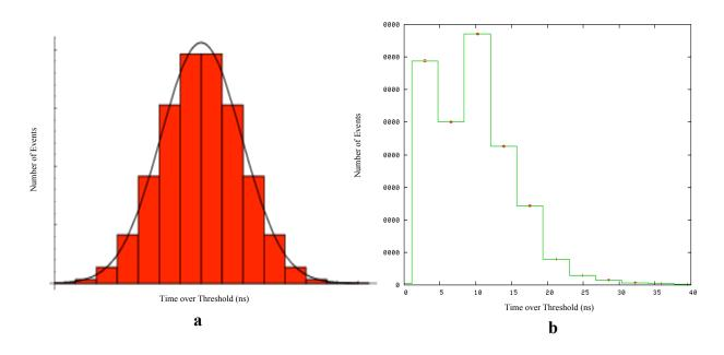
*Figure 18. (a) The Gaussian distribution expected from an 'ideal' system performance graph, (b) an actual system performance grph.*
