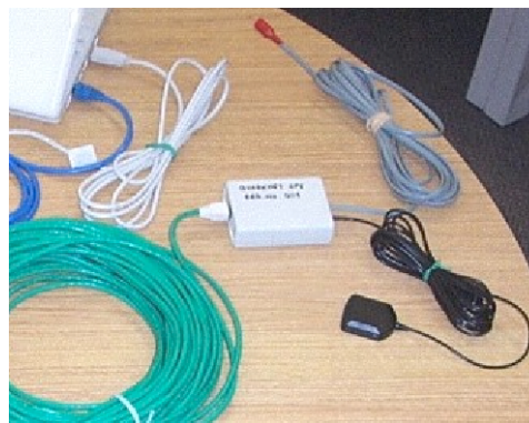
Figure 13. The GPS unit consists of a 100-ft. CAT-5 network cable (green cable), a GPS module (gray box), an antenna (black cable), and a temperature probe (gray cable, red end).
