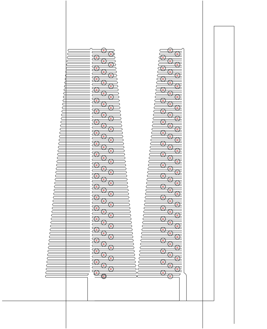
Figure 5: Footprint of the upilex Christmas-tree (horizontal lines) and the pins of the “bed-of-nails” probe.
