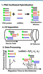
**Figure 1.** Schematic depiction of DQAMmiR with PNA hybridization probes.
