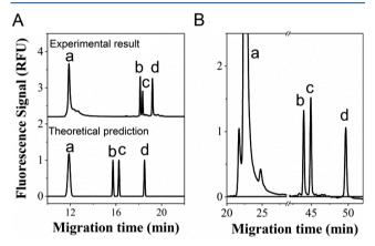
Figure 4. (A) Comparison of experimental and predicted separations of three PNA—miRNA hybrids in 20 mM Borax and 20% acetonitrile at pH 9.0. (B) Baseline separation of the three hybrids from each other by using a high-ionic-strength CE running buffer: 20 mM Borax, 120 mM NaCl, 20% acetonitrile, pH 9.0. Peak assignment: (a) excess PNA probes, (b) PNA-miR-147a (20 bp, 5 aa), (c) PNA-miR-378g (20 bp), and (d) PNA-miR-21 (22 bp).
