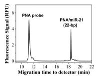
**Figure 2.** CE separation of a PNA probe from a PNA-miR-21 hybrid in a running buffer of 20 mM Borax and 20% acetonitrile at pH 9.0. The sample was prepared by incubating 2 nM miR-21 with a 10 nM PNA probe with a sequence fully complementary to miR-21. Separation was driven by an electric field of 312.5 V/cm at 20  $^{\circ}$ C.
