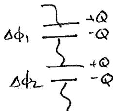
$$\Delta\phi = \Delta\phi_1 + \Delta\phi_2 = \frac{Q}{C} = \frac{Q}{C_1} + \frac{Q}{C_2}$$
