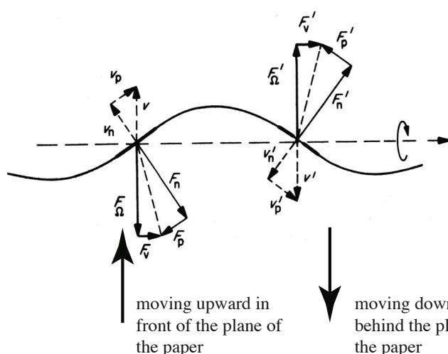
The velocities of each segment ( $v$ ) is decomposed into velocities normal ( $v_n$ ) and parallel ( $v_p$ ) to the segment. The frictional drag forces are also normal ( $F_n$ ) and parallel ( $F_p$ ). When  $F_n$  and  $F_p$  are decomposed into components normal and parallel to the helical axis, the net force  $F_v$ , contributes to the forward velocity<sup>[1]</sup>.
