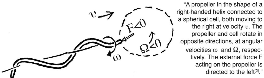
This can be simplified somewhat by removing the bacterial cell from consideration, leaving just the ‘propellor’, and revealing the combination of force and torque.
