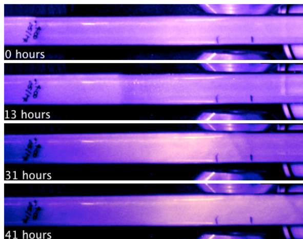
Figure 1. Experimental apparatus. Race tube containing the N. crassa colony under blue light. The edge of the colony can be seen marked on the left-hand side. The magnetic field is located between the two metal heads toward the right hand side. Colonies grew through the magnetic field so that growth before (0 and 13 hours), during (31 hours), and after (41 hours) magnetic field exposure could be monitored.
