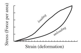
Experimentally, materials may be 'viscoelastic', leading to a stress-strain relation in which load and unloading of the force follow different paths of deformation.
