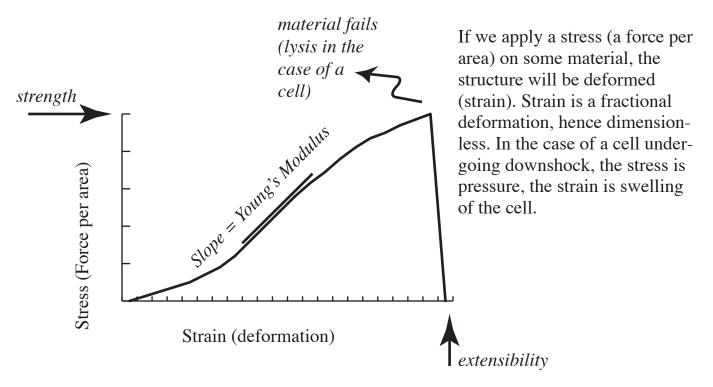
The steeper the slope (the greater the value of Young's modulus, in units of force per area), the stiffer (less deformable) the material.
