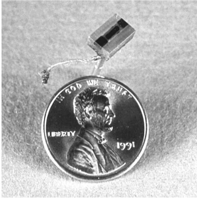
FIGURE 3. Old thermometer design. The central dark region is the exposed carbon.
