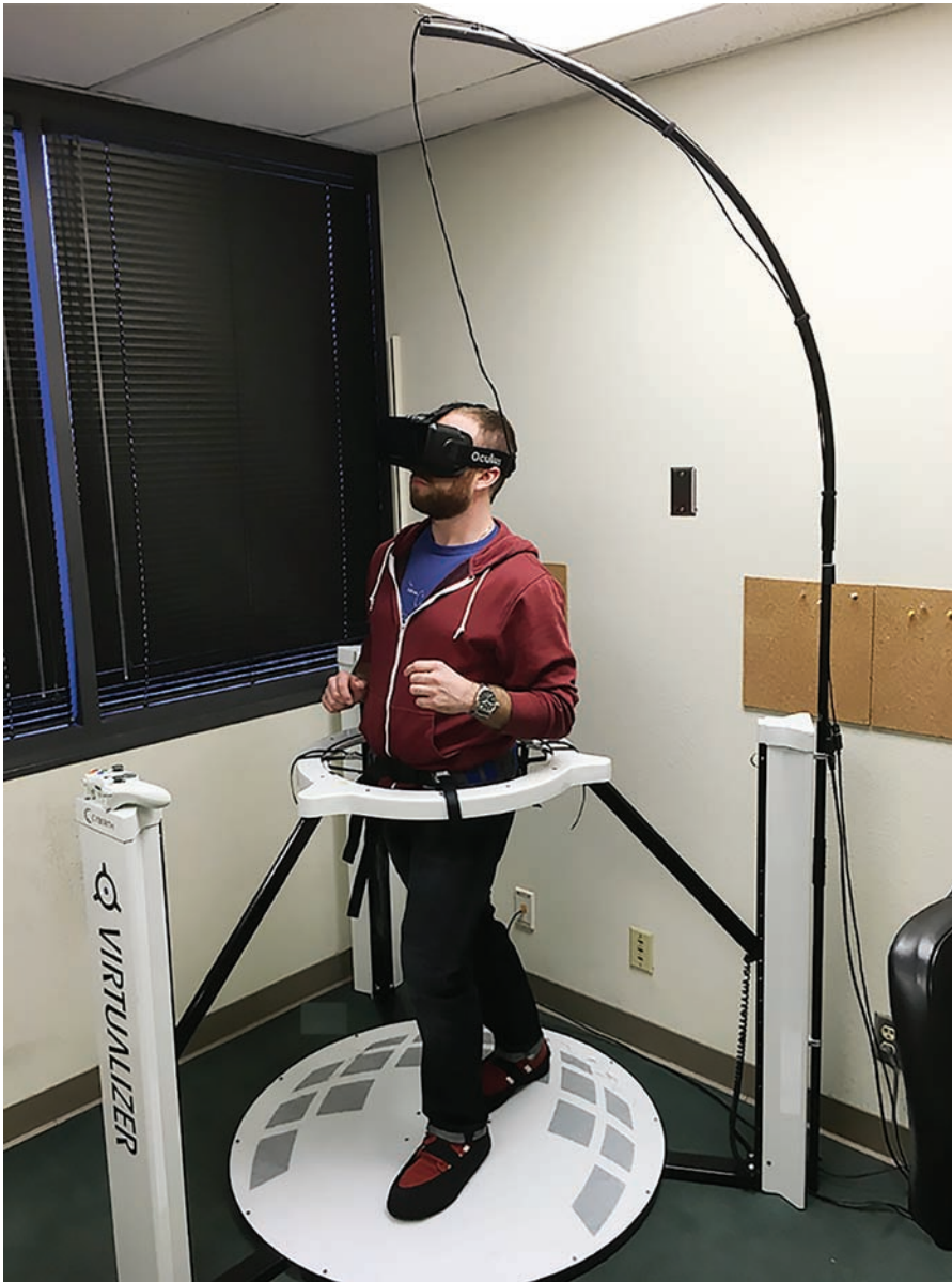
FIGURE 2.10. New tools to study human navigation. Example of an omnidirectional treadmill to test navigation in environmental space.
