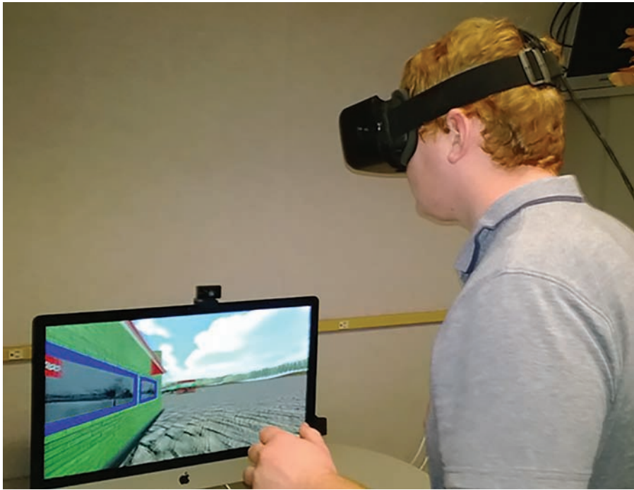
FIGURE 2.9. Using VR to study human navigation. A head-mounted display provides peripheral visual input and stereoscopic vision.
