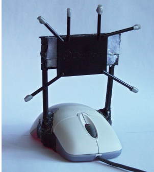
Figure 7. Mouse with optical tracking markers mounted.
