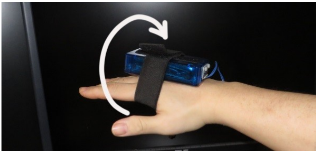
Figure 4: Extra IMU used for the twist selection method.
