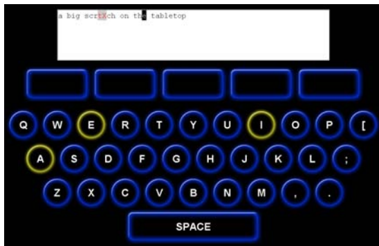
Figure 5. On-screen keyboard with letter prediction. The text phrase at the top is presented to the user for input.
