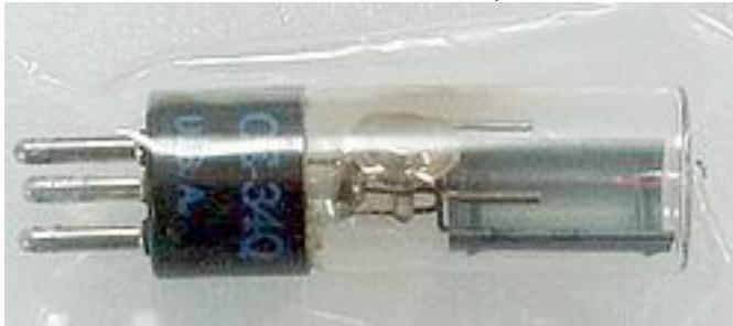
When light hits the surface an electric potential difference between post and mantle is measured.
