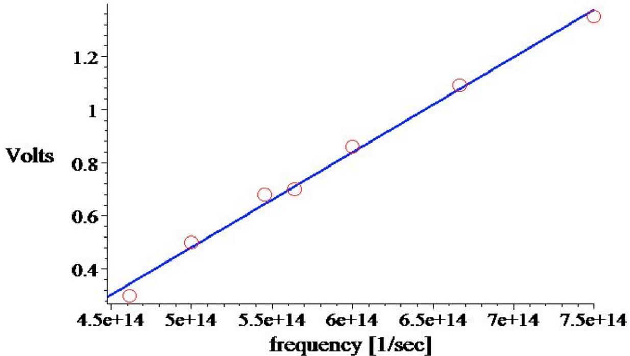
Fitted a line, read out the slope times **e**:
