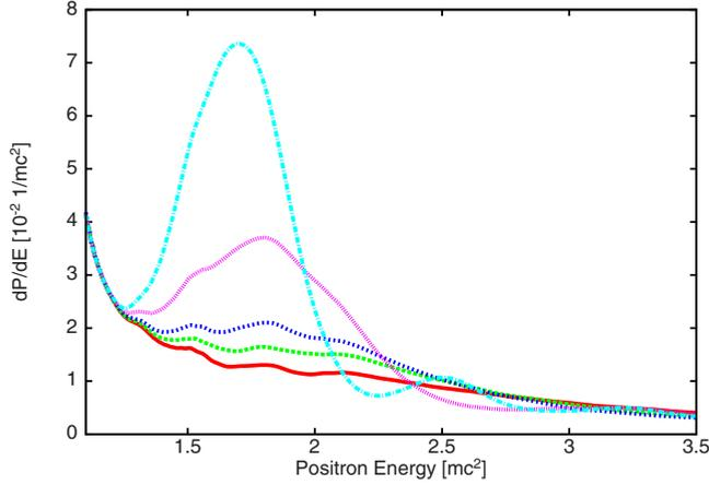
FIG. 3. (Color online) Total differential positron spectrum  $dP/dE$  for the U-U system at  $E_{c.m.}=740$  MeV, for different nuclear sticking times calculated using Eq. (2). The solid (red) curve is for  $T=0$ , the long-dashed (green) curve for  $T=1$ , the short-dashed (blue) curve for  $T=2$ , the dotted (magenta) curve for  $T=5$ , and the dash-dotted (cyan) curve for  $T=10$ .
