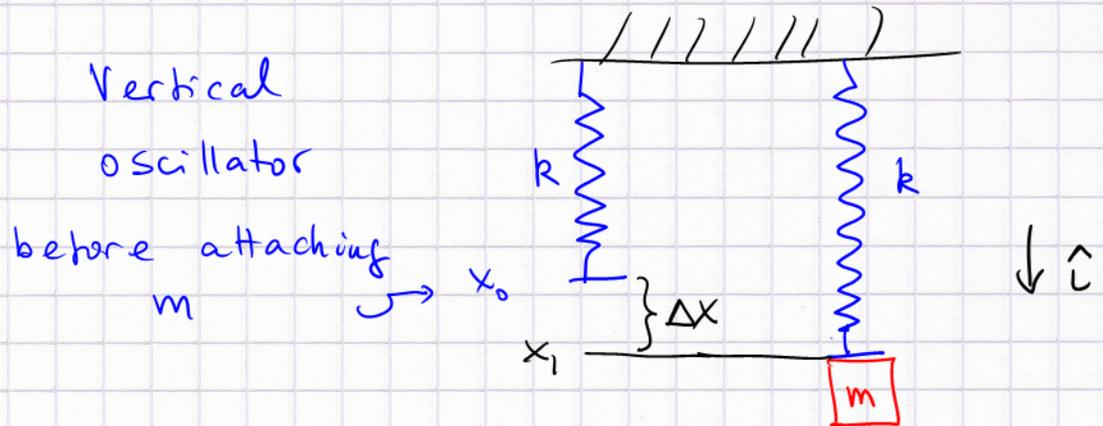
Step 1: figure out new equilibrium position  $x_1$  or its displacement  $\Delta x = x_1 - x_0$
