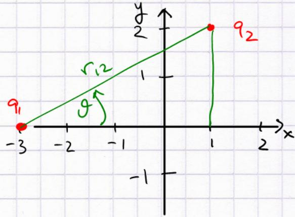
$$\begin{aligned} \text{The distance: } r_{12}^2 &= (x_1 - x_2)^2 + (y_1 - y_2)^2 \\ &= (-3.0 - 1.0)^2 + (0 - 2.0)^2 \\ &= 16.0 + 4.0 = 20.0 \text{ m}^2 \end{aligned}$$
