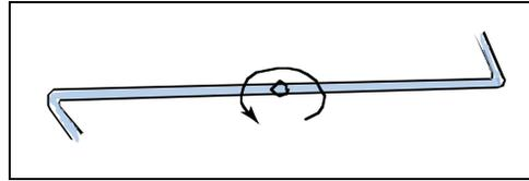
The force required to 'break' the water column at the center can be calculated from the angular velocity, radius, water density, and the area of the tube lumen. The data are shown in the figure. Maximal tensile strength is about 280 bars, equivalent to 28 MPa. Source: Briggs, LJ (1950) Limiting negative pressure of water. *Journal of Applied Physics* 21:721–722.
