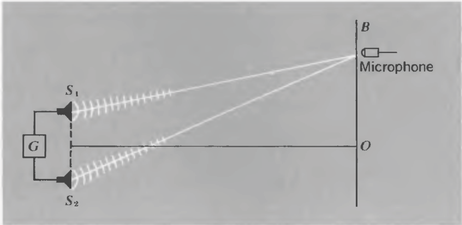
Fig. 2-2 Array to detect phase difference as function of microphone position in the superposition of signals from two loudspeakers.
