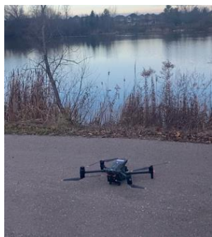
Drone used for thermal and ortho mapping
