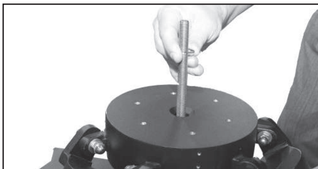
Figure D. Push the retaining clip onto the threaded rod.
