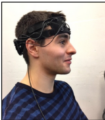
4th-year student in Biophysical Techniques course wearing a functional biophotonic cap which measures near-infrared absorption by hemoglobin to probe cerebral blood oxygenation changes.
